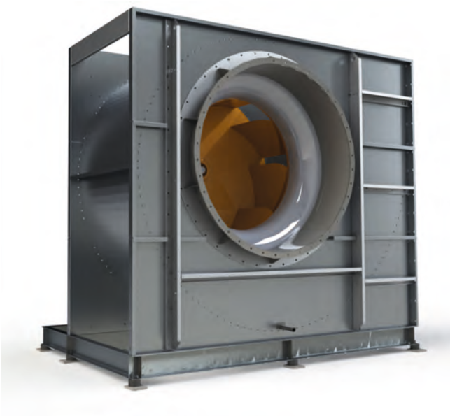
radial fan volume flows of up to 160.000 m 3 /h static pressure difference up to 3.000 Pa
